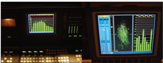
Figure 6.16 The A1 performing the mix has tools other than the ears. The display on the left is a spectral graph of an audio signal. It quantizes exactly how much bass and treble, along with the mid frequencies, a source has. The A1 can adjust how the audio mixer processes that signal. Many things can cause "roll-off" of low or high frequencies besides microphones, cabling or other electronic processing. Mic placement, combined with venue acoustics, can conspire to limit bandwidth. The display on the right is a graphical display of stereo, or multichannel separation. The object of multiple audio channels is to provide a 2-D (in the case of stereo) or a 3-D (in the case of additional channels) audio image. A mono audio feed would produce a single vertical line in the center of the display. Here audio channel separation is robust, providing a stereo image and not simply a single point of audio.
