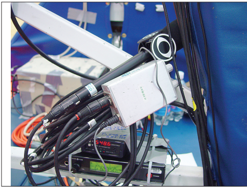
Figure 6.10 The people involved with audio setup have to be concerned with not only with sound acquisition, but also with the distribution of the communications gear necessary for the production. Here a reporter's package of microphone and intercom/IFB is placed near a basketball court where it will be used during the show.
