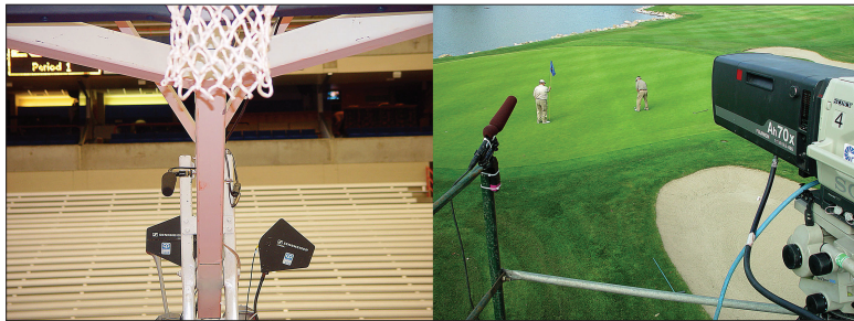
Figure 6.10 The people involved with audio setup have to be concerned with not only with sound acquisition, but also with the distribution of the communications gear necessary for the production. Here a reporter's package of microphone and intercom/IFB is placed near a basketball court where it will be used during the show.
