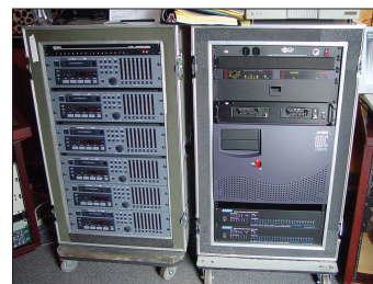
Figure 6.14 Each multitrack (multichannel) recorder, on the left, records eight tracks of audio, allowing the whole case of recorders to handle 48 tracks.
