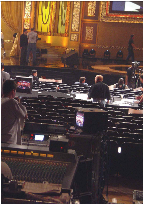
Figure 6.15 All mixes are different, even ones done at the same venue at the same time. For instance, the audio people creating the mix for the PA feed in the house (shown above) will mix the show differently than the audio folks outside in the television production trucks, even though they are using many of the same sources.
